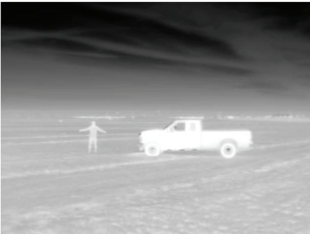
**FIGURE 5: HUMAN AND VEHICLE SHOWN AT 25 METERS AND 40° FIELD OF VIEW USING AUTOMATIC GAIN CONTROL**
