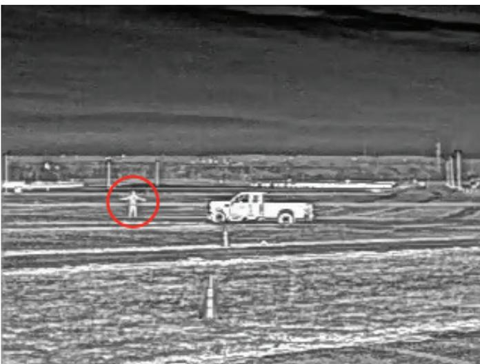
**FIGURE 4: IMAGE OF HUMAN AT 100 M USING 19 MM FOCAL LENGTH 320 x 240 IMAGER HAVING 16° HORIZONTAL FIELD OF VIEW**
