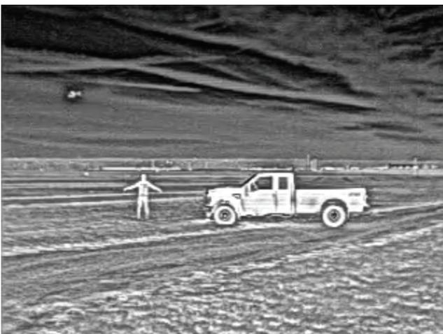
**FIGURE 6: HUMAN AND VEHICLE SHOWN AT 25 METERS AND 40° FIELD OF VIEW USING IMAGE CONTRAST ENHANCEMENT (ICE™)**
