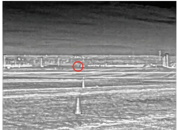
**FIGURE 3: IMAGE OF HUMAN AT 1000 M USING 19 MM FOCAL LENGTH 320 x 240 IMAGER HAVING 16° HORIZONTAL FIELD OF VIEW**
