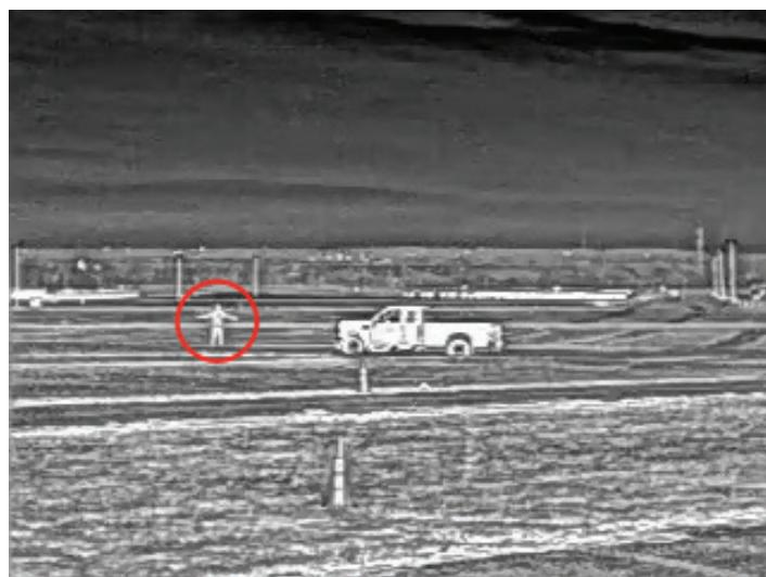
FIGURE 4: IMAGE OF HUMAN AT 100 M USING 19 MM FOCAL LENGTH
