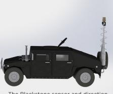
The Blackstone sensor and direction finding (DF) antenna head are easily repurposed from their soldier-worn configuration to a vehicle configuration in less than five minutes.
