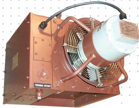
Unit Heaters are designed for overhead mounting. The units consist of a fan and motor, steam/hot water heating coil, fan guard and directional louvers built as a single unit. Electric heating elements are available in lieu of the standard steam/hot water coil.
