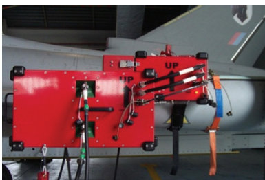
DRS RF hoods enable accurate characterisation and measurement of EW system performance
