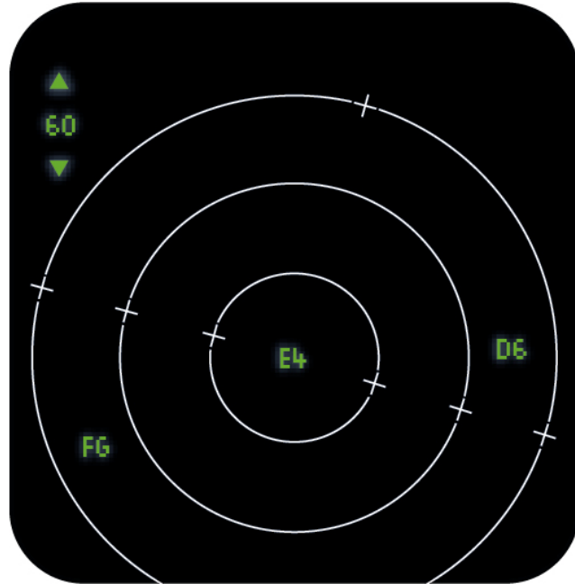
Fig 1. This display indicates the type of signal that might be received by the platforms EW system. The position of the TAG represents the signal position relative to platform and its signal strength.
