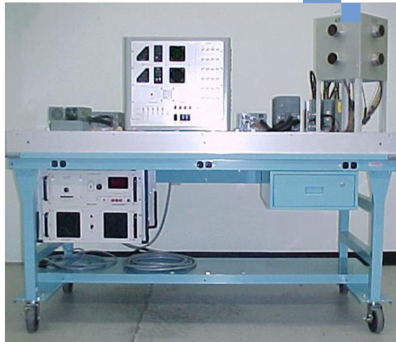
Hot Mock-up Bench paired with a DRS Antenna Coupler Set and a DRS Electronic Combat End-to-End Tester (ECETET).
