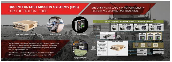
The multi-faceted DDU gives the mobile user a host of bundled and on-the-move capabilities. They comprise a rugged latest-generation PC, a data router, a multi-OS server, a tactical LTE host, a GPS distributor, a data recorder, a video-management device, and a communications crossbanding solution.
