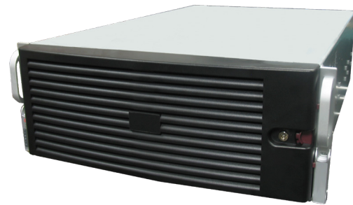
A 4U 19-inch rackmount configuration weighing approximately 100 lbs.
